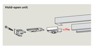
The **RF** mechanical hold-open unit ensures that doors are held open at precisely the correct angle – up to approx. 150° – without any fallback.
