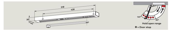
The **G-EMF** slide channel assembly enables the door to be held open securely at a preselected position without fall-back. The hold-open point can be adjusted within an opening angle of approx. 80° and 140°.
