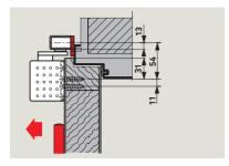
**Mounting backplate 30 mm for G-N**For fixing the slide channel to the door frame where there is no means of direct mounting.
