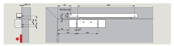
**TS 92 B** closer with G-EMF slide channel assembly, pull-side fixing Example: Anticlockwise-closing (ISO 6) door; mirrored arrangements apply to clockwise-closing (ISO 5) doors.
