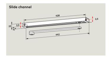
The **G-N** slide channel assembly comprises the main arm, slide channel, slide block, fixings, screws and end caps. The G-N slide channel is non-handed and can be combined with both door closers.
