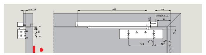
**TS 92 G** closer with G-EMF slide channel assembly, push-side fixing Example: Anticlockwise-closing (ISO 6) door; mirrored arrangements apply to clockwise-closing (ISO 5) doors.
